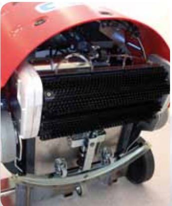
The robo 40 is a full-fledged scrubber dryer with 2 cylindrical brushes and a suction nozzle
