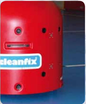
The robo 40 navigates itself with the help of 8 ultrasonic and 4 infrared sensors
